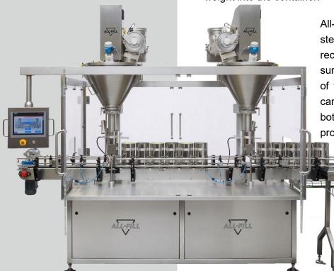
All-Fill's unique conveyor chain, stainless steel or plastic as appropriate, provides a recess-free wipe-clean stainless steel surface and affords access to the underside of the container for lifting. Neck locators can be utilised for centralising narrow-neck bottles, and vibration settling for granular products.
