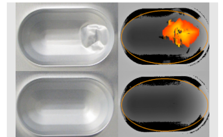
Photo and evaluation view of blister inspection
