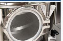
+ Inspection windows in the deduster housing for optimum viewing of the product area during the dedusting and conveying process
