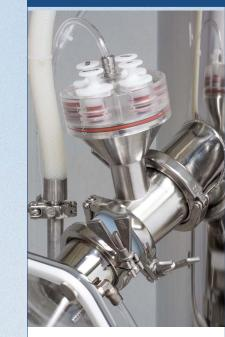
+ The test tablet dispenser KT2010 is an innovation that allows for easy contained metal detector sample tablet insertion without breaking containment
