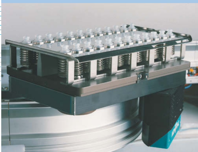
Transport shuttle: Transporting the cartridges in a shuttle using a rail system
