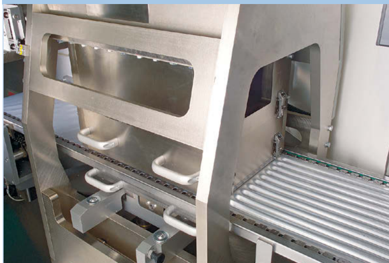
Cool indeed: Cold forming of the catheter package
