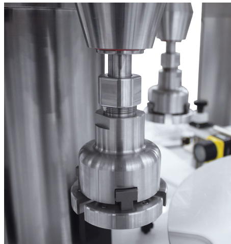
Pick & place system with gripper chuck for unique cap applications.
