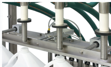
Pressure, vacuum or gravity level filling.
