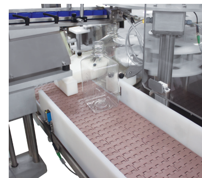
Positive reject system on conveyor.
