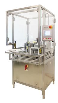
The operator inserts a syringe nest into the nest carrier and then starts the filling process via the touch screen HMI. The FSV will automatically locate the syringe underneath the filling needle and lower the needle into the container. The FSV flushes the syringe with nitrogen before it starts the filling process automatically. Simultaneously to the filling process a rubber stopper is placed into the
