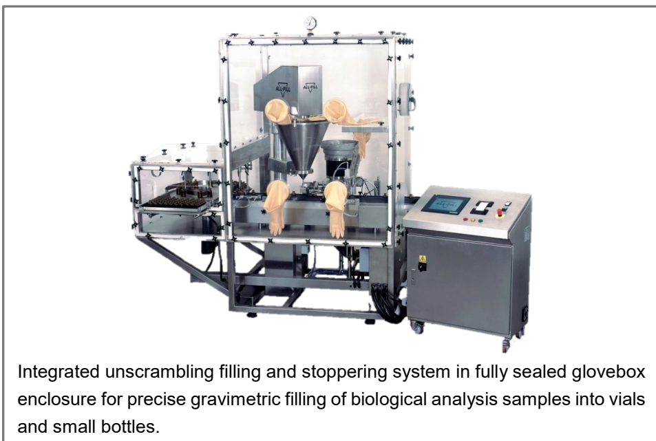
Series 1 Micro-Fill unit for laboratory and production use. 10mg to 50g. Inclusive of servo drive, colour touch-screen HMI and integral workstation.
