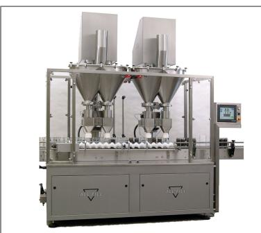
Series 400 quad-head in-line filler for filling instant coffee into round and square glass jars and tin cans. Features include wormscroll container feed, flex-seal dust control, volumetric filling of instant coffee powder, gravimetric filling of freeze-dried and agglomerated coffee, container vibration for granular settling.
