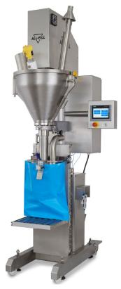
Larger fill weights or inconsistent products demand a gravimetric approach for improved accuracy and reduced give-away. The Series 10 Sack filler can fill pails and sacks up to 25kg. The pneumatic bag clamp ensures that sacks are held securely during filling but can be removed tool-free when pails are being filled.
